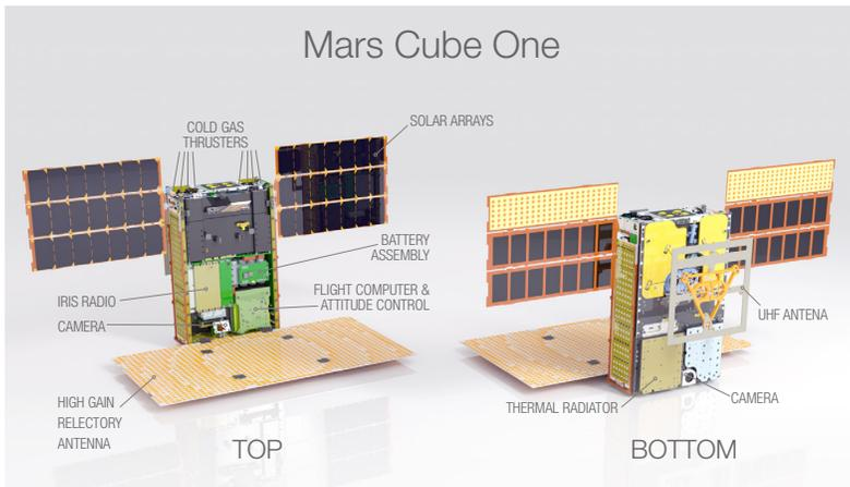
Illustration of the twin MarCO spacecraft with some key components labeled. The top cover is left out to show some internal components. Antennas and solar arrays are shown deployed.
