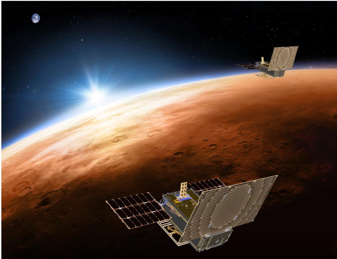
*An artist's rendering of the twin MarCO spacecraft flying over Mars with Earth in the distance. The MarCOs are the first CubeSats, a kind of modular mini-satellite, to fly to deep space. They were designed to fly along with NASA's InSight lander on its cruise to Mars. Should they make it all the way to Mars, they will provide relay of data about InSight's entry, descent and landing back to Earth.
